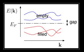
Usually an energy gap separates the filled valence bands from the empty conduction bands. The  $Fermi\ level\ E_F$  characterizes the gap.
