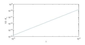
The numerical solution also indicates other properties, for instance, that the first eigenvalue behaves as  $\epsilon_1 = \frac{1}{2} - c\lambda^4 + o(\lambda^4)$  as  $\lambda \to 0$ , with  $c \approx 0.0156$ .
