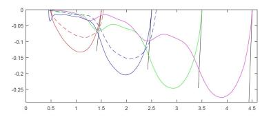
Resonance trajectories as  $\lambda$  changes for zero to  $\sqrt{2}$ . The weak-coupling asymptotes are shown. The 'non-threshold' resonances at the second and third sheet appear at  $\lambda=1.287$  and  $\lambda=1.19$ , respectively.
